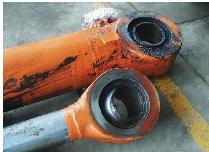
Bearings at hydraulic cylinders of a hydraulic excavator
